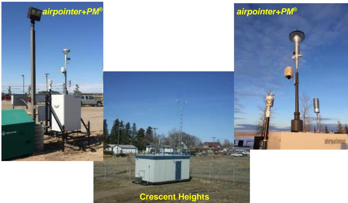
**Figure 2. PAS Continuous Air Quality Monitoring Stations**
