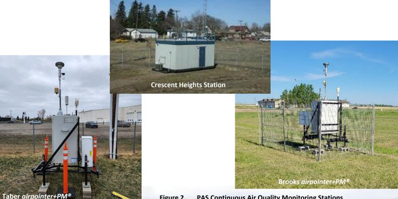
Figure 2. **PAS Continuous Air Quality Monitoring Stations**
